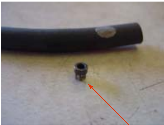
This is a picture of an EGR flow orifice. As you can see, it resembles a carburetor jet.
