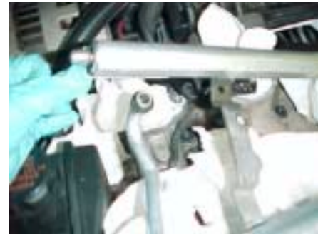
View with crossover tube removed and o-ring exposed
