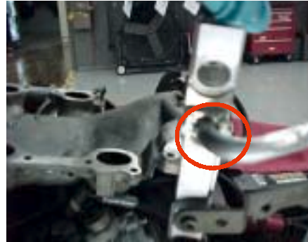
Bottom side of the rear portion of the fuel rail where the crossover tube fits.
