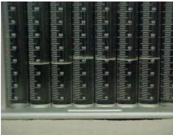
(Picture 2: actual fuel volume as tested on our flow bench)
