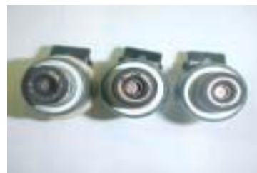
Carbon build-up reduces flow
