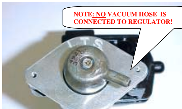
FIGURE # 6 INSTALL RETAINER WITH LTS OUTWARD.
